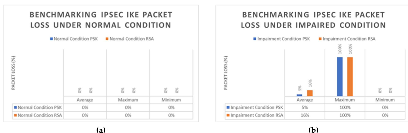
Figure 7. Packet Loss: (a) in normal conditions, (b) in impaired condition
