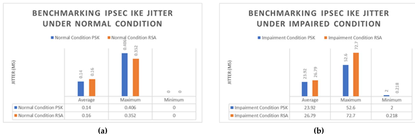
Figure 6. Jitter: (a) in normal conditions, (b) in impaired condition
